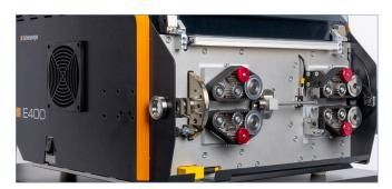
Different feed belts and coatings of the rollers ensure optimum transport of the cables. The contact pressure on the feeding unit is programmable. The E400 is equipped with a belt drive with integrated short piece kit.
