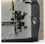
Different feed belts and coatings of the rollers ensure optimum transport of the cables. The contact pressure on the feeding unit is programmable. The E300 is equipped with a two-in-one quick-change feeding unit suitable for roller drives, including a short piece kit for the processing of short cables.
